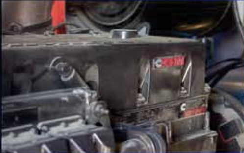
Cummins QSM Tier 3 /4i Engines meet Strict Emission Standards
